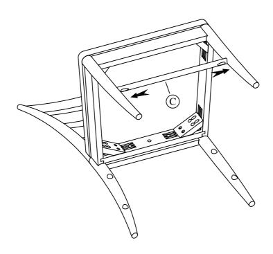
STEP 5: Attach Side Stretcher (Top), no need to attach Screws.
